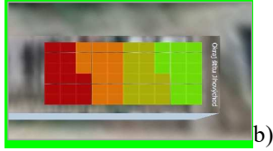
Fig. 5. The connection of panels into 4 strings for 3rd variant.
